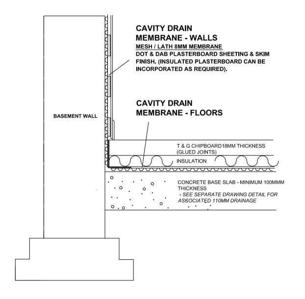
FOR DRAINAGE DETAIL REFER TO BLG DRAWING 005 -CENTRAL DRAINAGE TO SUMP
